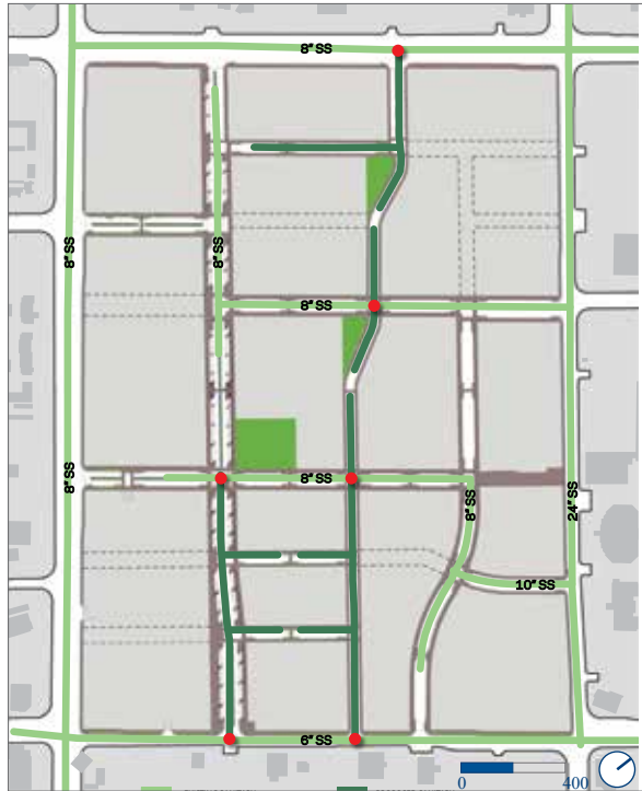
Exhibit 2.34: Proposed Sanitary Sewer System Map
